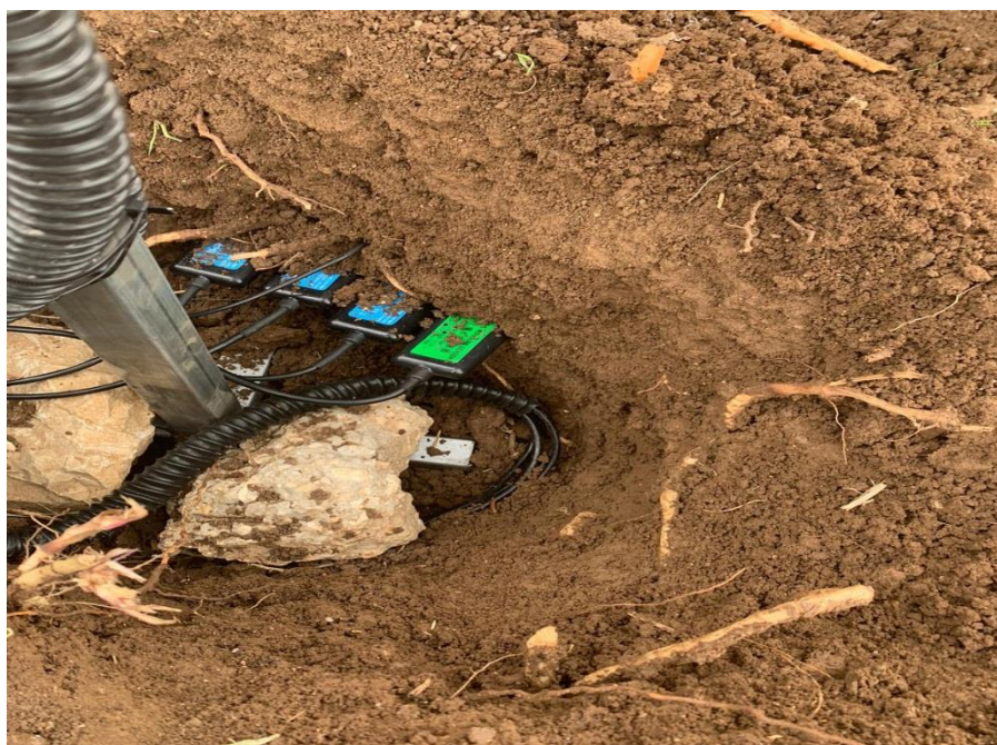
Figure 8: Insulation of sensors in the soil
