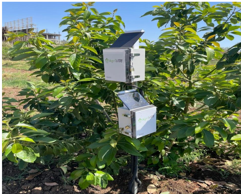
Figure 7: Smart system for measuring N-P-K in the open orchards field
