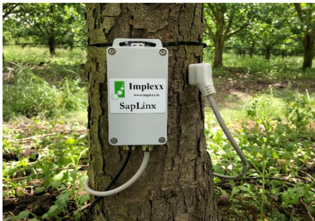
Figure 4. Sap flow sensor probe (right) and data logger on a pear tree. (Edaphic Scientific), https://edaphic.com.au/products/sap-flow-sensors/multi-sensor-sap-flow-system/
