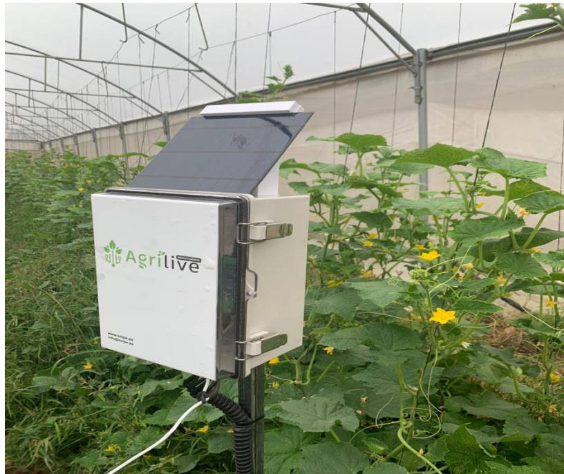
Figure 6: Smart system for measuring N-P-K in the greenhouse
