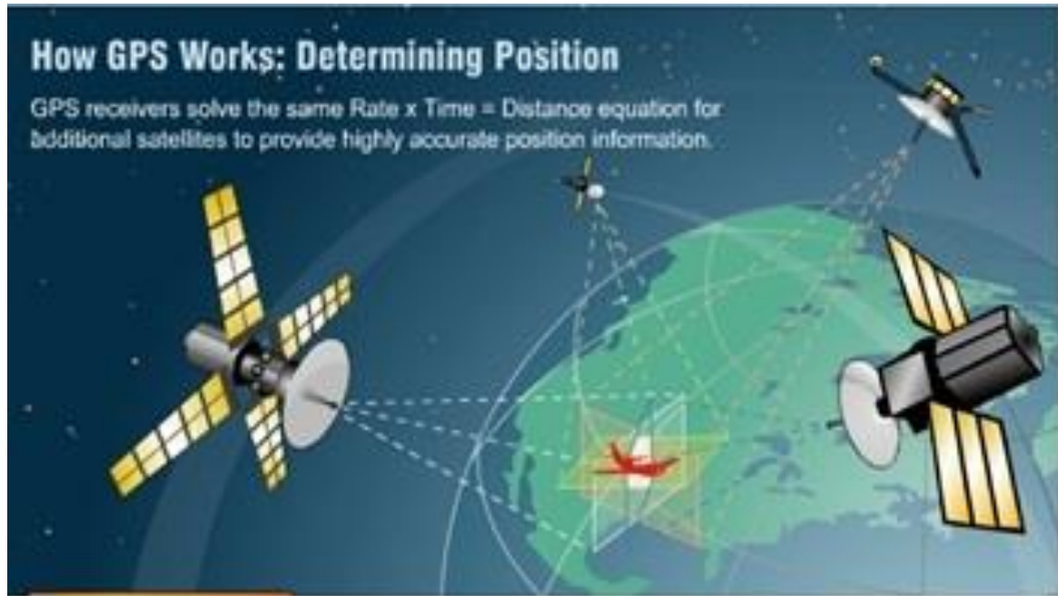
Figure 3. Global positioning system (GPS) and working
