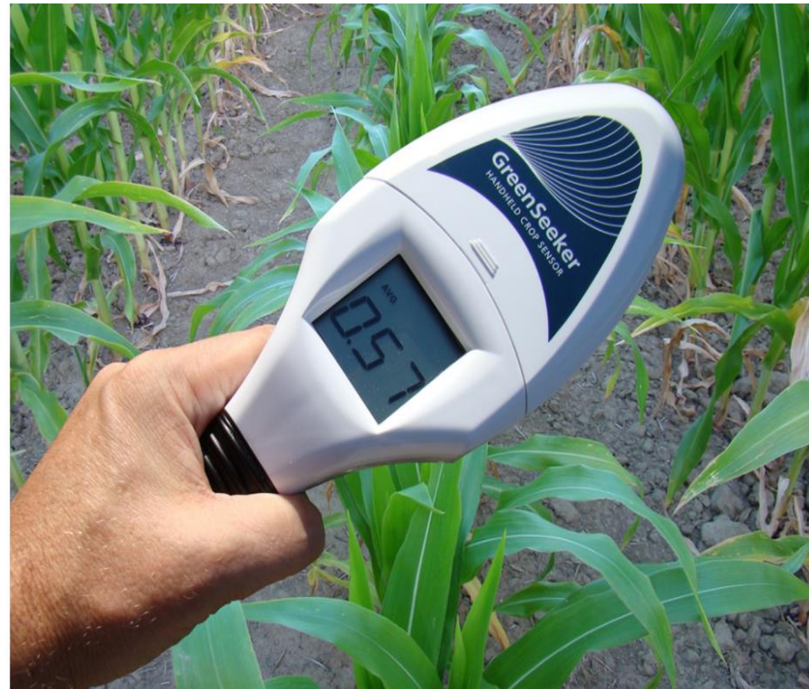
Use of sensors green seeker under field conditions
